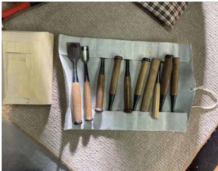
Chisels used for the initial rough carving (or striking the mask). | Photo by Udaka Keiko, Instagram.
